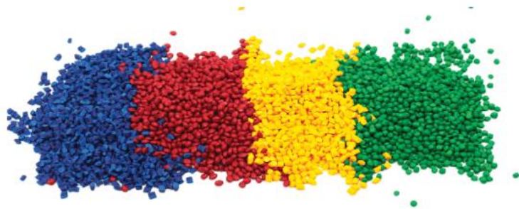
Figure 21.30 Plastic pellets obtained from the physical method of recycling
