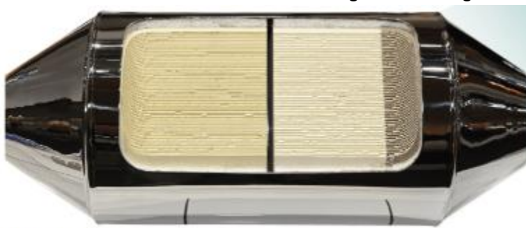
Figure 22.6 The internal honeycomb structure of a catalytic converter
