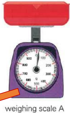
▲ Figure 1.34 Weighing scales showing different readings when nothing is placed on them
