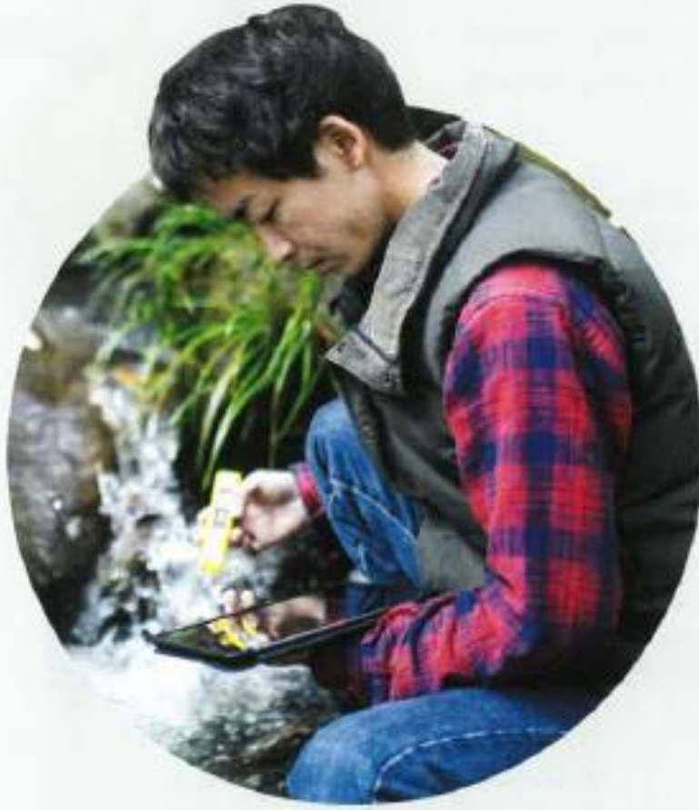
▲ Figure 1.5 Scientist using a data logger to collect real-time data of a water body
