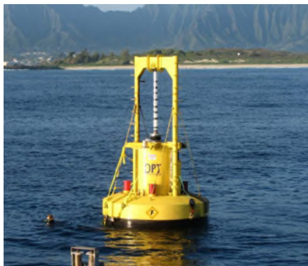
Rise and fall of a buoy generates 20 kW.
