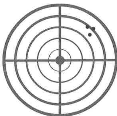
▲ Figure 11 Precision — In this figure, the points are precise because they are clustered at the same place, but far from the actual value (indicated by the dot ●).
