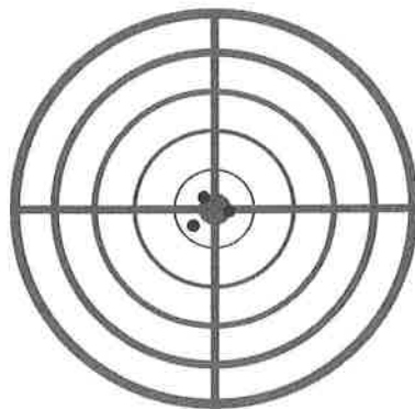
▲ Figure 13 Accuracy and Precision — In this figure, the points are close together and near the actual value. Hence, they are precise and accurate.
