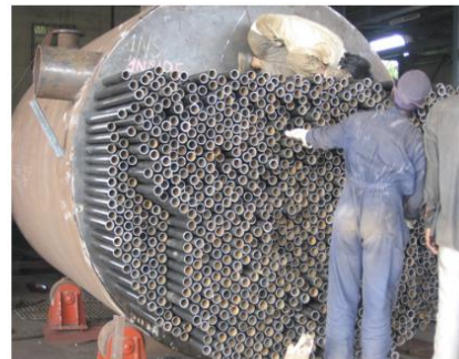
Tubes in a heat exchanger
