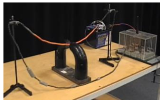
Fig. 3.1 Fleming's Left-Hand Rule
