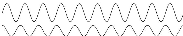
Fig. 11.16 Two sound waves (different amplitudes) with a phase difference of \pi/2 is coherent.
